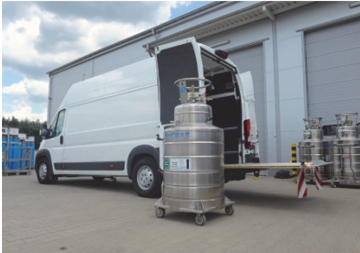
Photo 2. A delivery truck with a tank for the transport of liquid helium
