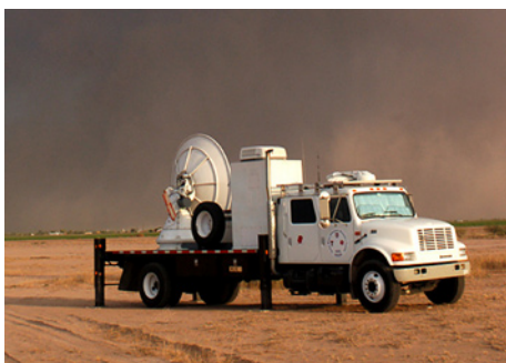
Fig. 11. Mobile weather radar
